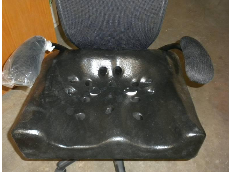
Figure 7 – OBSS chair assembly with breather holes.
